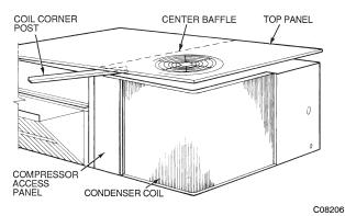
Fig. 9 - Propping Up Top Panel
